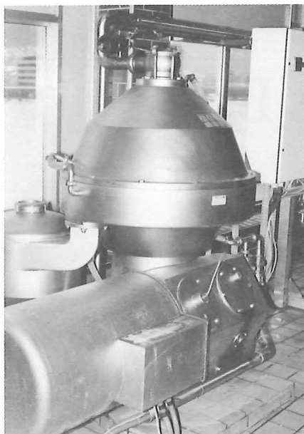
Beer centrifuge in the filter room at Aass Brewery.
